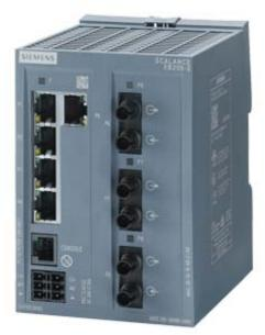
Preset for PROFINET mode! SCALANCE XB205-3 managed Layer 2 IE Switch 5x 10/100 Mbit/s RJ45 ports 3x MM FO ST-Port 1x console port, diagnostics LED redundant power supply; temp. range 0 °C to +60 °C; mounting onto standard rail; Default PROFINET
